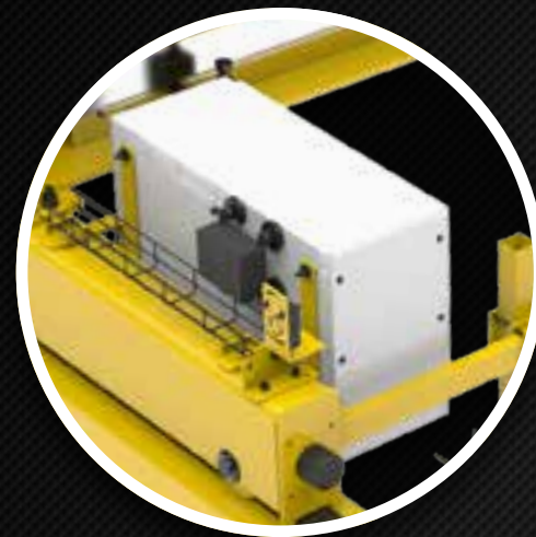
Control panel with receiver
